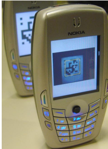
Figure 5.3: SiB application on a Nokia 6620 with one phone scanning a barcode on the LCD of another.
