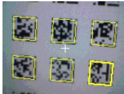
Figure 5.4: Mobile phone screen shot showing the SiB application on a Nokia 6620 recognizing multiple tiled barcodes displayed on an LCD screen.
